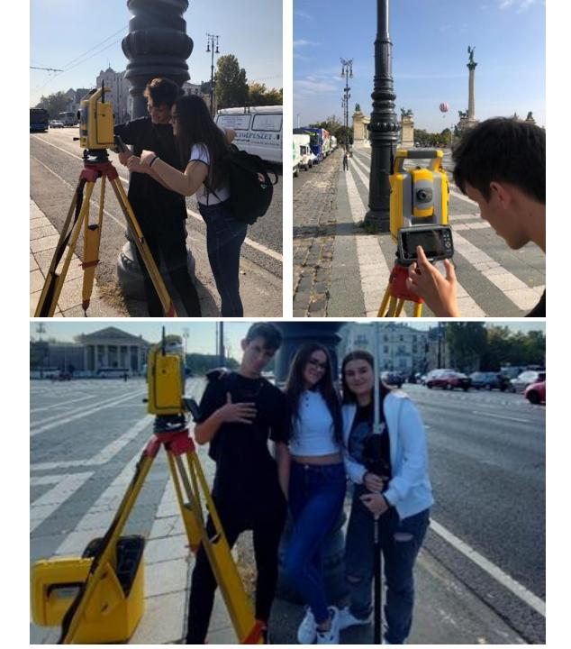
• Entering values from measurements with a GPS receiver into the Total station (Y, X, altitude)
